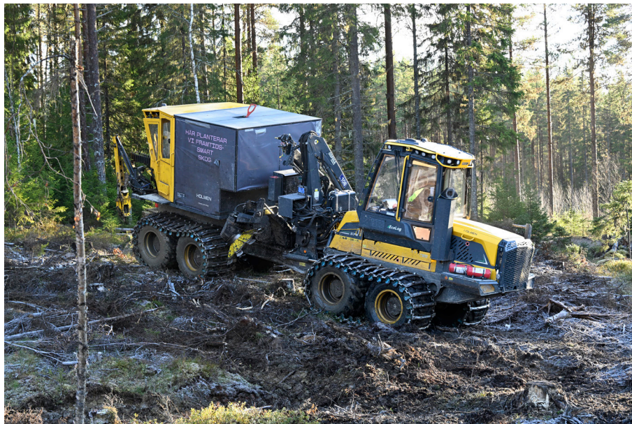
Fig. 1. PlantMax planting machine built on Eco Log 574E forwarder, equipped with a MidiFlex disc trencher. Photo Mikael Rönqvist.
