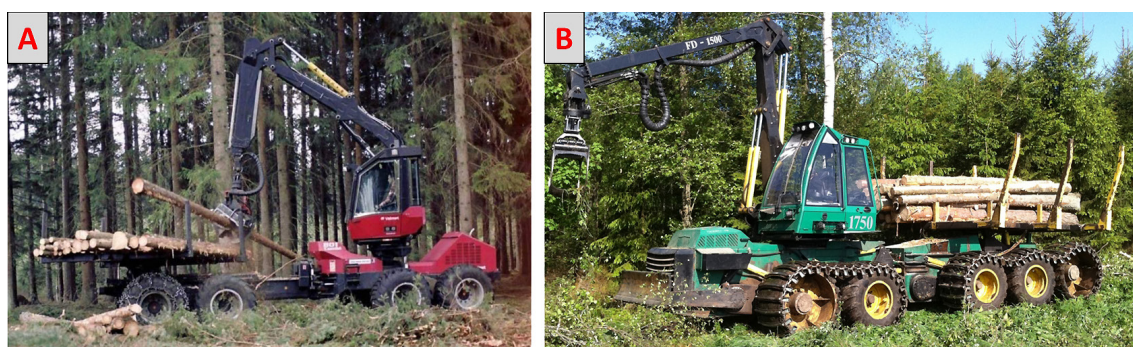
Fig. 3. Rotatable and tiltable load spaces/bunks on previous SMS (Valmet 801 Combi harwarder and Fibredrive 1750). These types of bunks allow for efficient direct loading, efficient unloading, and semi-automation on SMS. Photos: Skogforsk (A) and Back Tomas Ersson (B).
