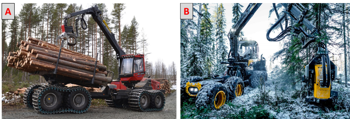
Fig. 1. Previous examples of large single-machine systems (LargeSMS): A) harwarder (Komatsu X19 prototype during unloading using a loading grapple); B) dual machine (Ponsse Buffalo Dual in harvester mode). A harwarder processes the logs directly onto the machine's load space (termed direct loading), while a dual machine initially works as a normal harvester and processes the logs into piles on the ground. Thereafter, the dual machine converts into a forwarder, loads the logs from the ground, and forwards them to the landing. Photos: Rikard Lundqvist (A) and Ponsse Plc (B).
