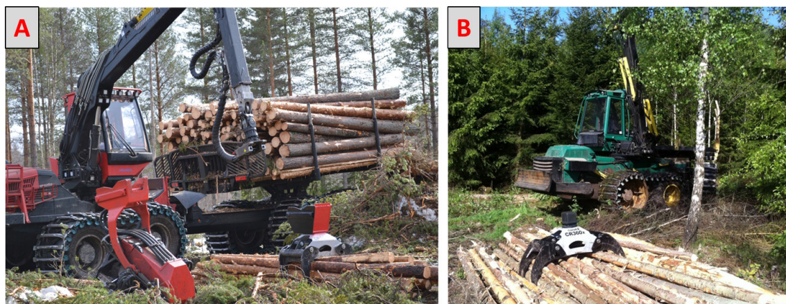
Fig. 2. Examples of quick coupling technology on: A) the Komatsu X19 harwarder prototype and; B) the Fibredrive 1750 harwarder prototype. Quick coupling technology increases the competitiveness of single-machine systems (SMS) compared to two-machine systems (TMS) by reducing the time needed to switch between harvesting heads and loading grapples on both harwarders and dual machines. This reduction in time consumption allows for more efficient work methods and/or raises the SMS' machine utilization. Photos: Rikard Lundqvist (A) and Back Tomas Ersson (B).
