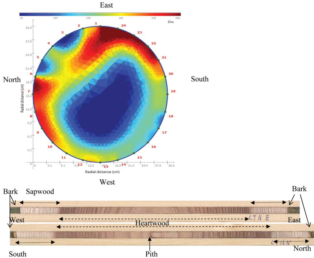
**Fig. 7.** Electric resistivity (ER) tomographic data and increment core with a non-centralized pith of Japanese cedar (*Cryptomeria japonica* D. Don) at a position of the detected cross-section (no. CJ16).
