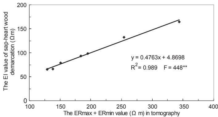
**Fig. 5.** Relationship between the maximum ER plus minimum ER (ERmax + ERmin) values and the corresponding electric resistivity (ER) value of the sapwood-heartwood demarcation (of an increment core) of the tomographic data (Taiwania (*Taiwania cryptomerioides* Hayata),  $n = 7$ ).
