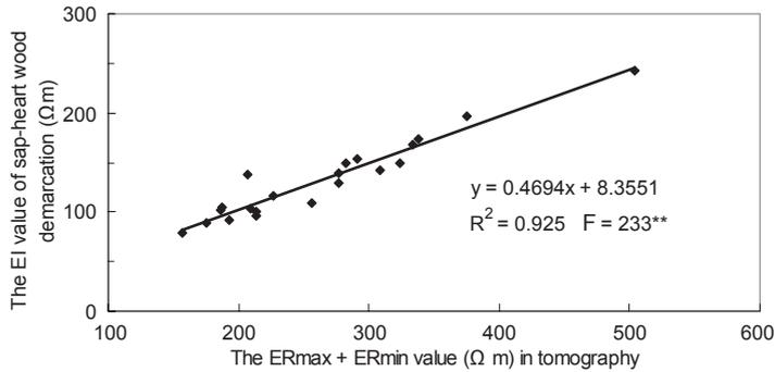
**Fig. 4.** Relationship between the maximum ER plus minimum ER (ERmax + ERmin) values and the corresponding electric resistivity (ER) value of the sapwood-heartwood demarcation of the tomographic data (Japanese cedar (*Cryptomeria japonica* D. Don),  $n = 21$ ).
