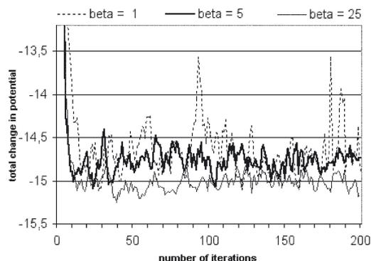
**Fig. 5.** Convergence of the simulation method with three different values of  $\beta$ . One iteration means 25 move attempts. The y-axis shows the total change in potential from the initial structure.
