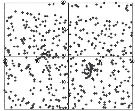
Fig. 7. A positive site potential on the low left and up (a forest road). Two negative point potentials close to each other in the middle.
