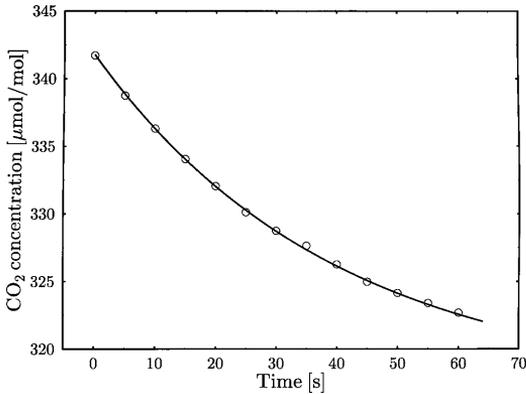
**Fig. 2.** An example of one series of daytime  $\text{CO}_2$  concentration measurements inside a closed cuvette at Värriö. The curve is obtained by exponential fitting with constant conductance assumption.
