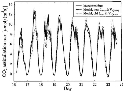
**Fig. 8.** CO<sub>2</sub> assimilation rate during 16.–23.7 1996 in Värriö cuvette 0 according to measurements and biochemical model with two different temperature dependences for  $V_{c(max)}$  and  $J_{max}$  (Table 3). Irradiance parameters  $q$  and  $\Theta$  and substomatal concentrations of CO<sub>2</sub> and O<sub>2</sub> were estimated from measurements. Fluxes are 60 min. averages.
