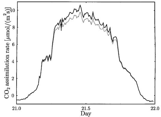
**Fig. 3.** The  $\text{CO}_2$  assimilation rate during 20.7.1996 in Värriö as estimated by two methods: Solid line: Constant conductance assumption in exponential fitting.  $g'_c$  was multiplied with first concentration in a closed cuvette to obtain the flux. Dotted line: Constant flux assumption in exponential fitting.
