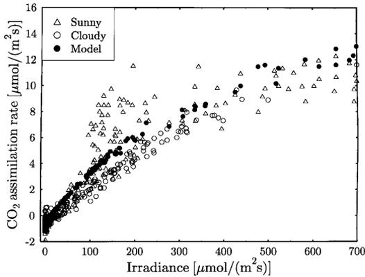
Fig. 6. The irradiation dependence of the CO<sub>2</sub> assimilation rate according to the biochemical model and measurements during bright and cloudy mornings. Fluxes are scaled to 15  $\mu\text{mol}/(\text{m}^2\text{s})$ .
