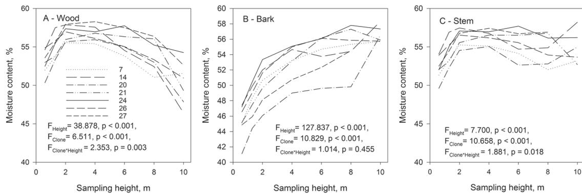
**Fig. 5.** The mean moisture content of wood (A), bark (B), and stem (wood and bark) (C) of the studied hybrid aspen clones at different sampling heights.
