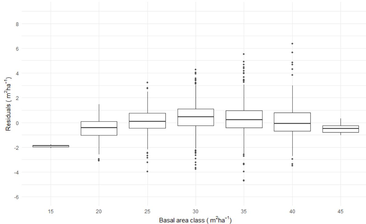
Residuals versus predicted values of the total basal area development function (BA1) fitted for the validation data set containing data from 12 silver birch thinning experiments in Finland.
