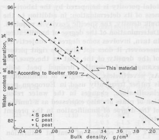
Fig. 16. Dependence of the water content of peat at saturation on its bulk density.
