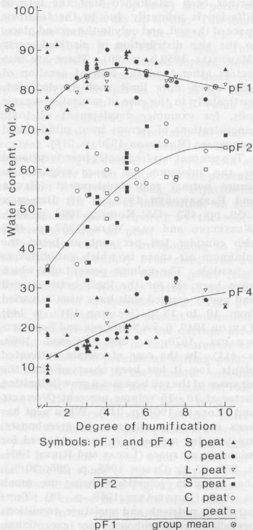
Fig. 20. Relationships between the quantity of water retained in peat at matric suction of pF 1, 2 and 4 and its degree of humification.
