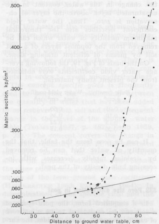
Fig. 23. Tensiometer recordings on the matric suction of sedge peat 5–10 cm below the ground surface at different depths of the ground water table. The unbroken line indicates the theoretical matric suction, the broken line having been obtained by fitting the actual recordings by hand.
