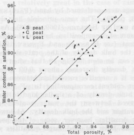
Fig. 17. Relationship between the water content of peat at saturation and its total porosity on the basis of the present material (unbroken line) and theoretically (broken line).
