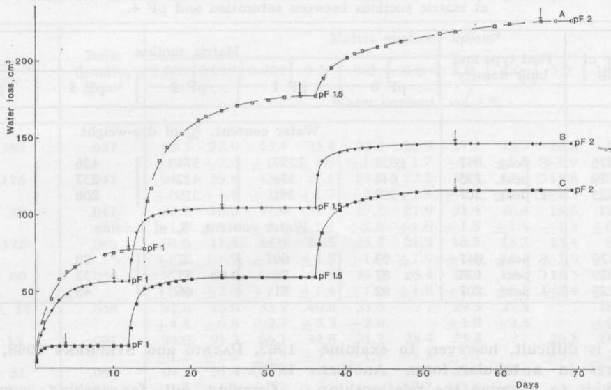
Fig. 14. Time required to reach equilibrium in pressure cell determinations. A = Sample 188, bulk density 0.056; B = Sample 153, bulk density 0.091; C = Sample 152, bulk density 0.155.
