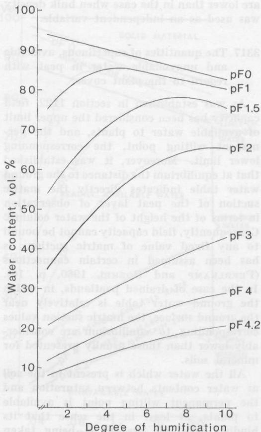
Fig. 21. Relationships between the quantity of water retained in peat at various matric suction and its degree of humification.
