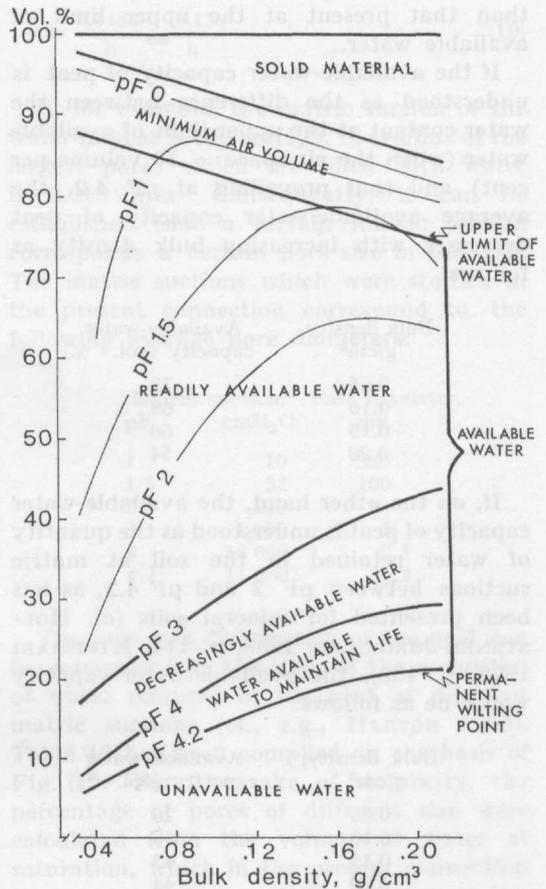
Fig. 22. Volumes of solid material and minimum air space as well as of water available (readily available + decreasingly available + available to maintain life) and unavailable to plants in peats with different bulk density. The thin lines show the quantities of water retained in the peat at pF 0, 1, 1.5 and 2.
