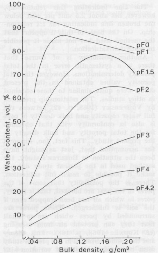
Fig. 19. Relationships between the quantity of water retained in peat at various matric suctions and its bulk density.
