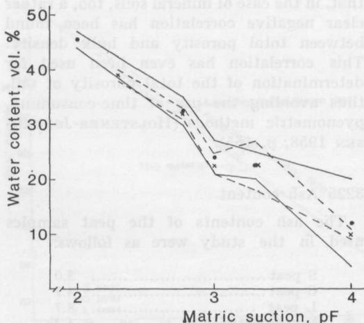
Fig. 13. Results from water retention determinations in a thermostat room (indicated by •; confidence interval indicated by unbroken line) and under normal laboratory conditions (indicated by × and broken line respectively).
