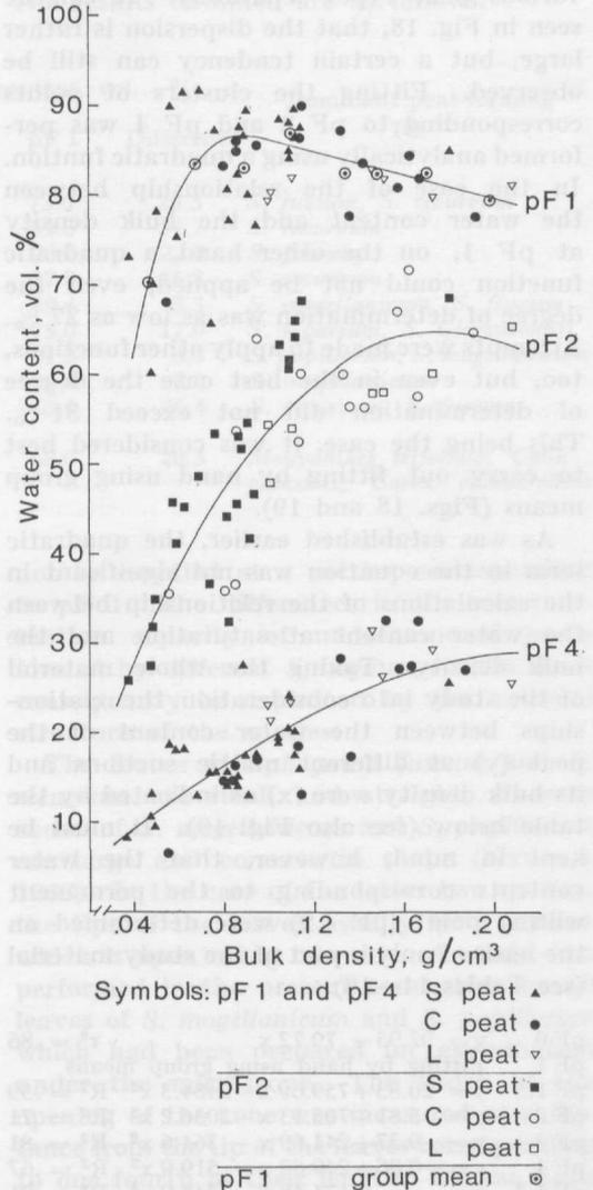
Fig. 18. Relationship between the quantity of water retained in peat at matric suction of pF 1, 2 and 4 and its bulk density.
