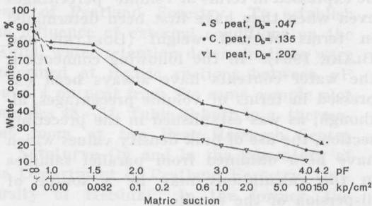
Fig. 15. Water desorption characteristics for different peat types ( $D_b$  = bulk density).
